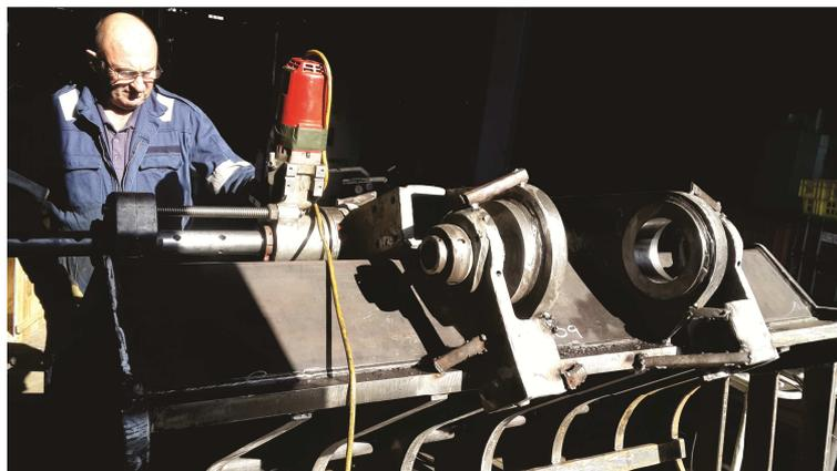
*Figure 3: Onsite machining of Excavator buckets*
